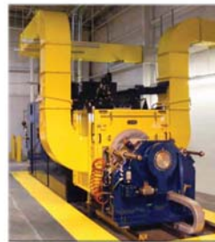
Webb's Link dyno simulates vehicle brake performance in an accelerated yet controlled laboratory environment. Data collected here empowers Webb engineers to develop products with improved performance and durability.
